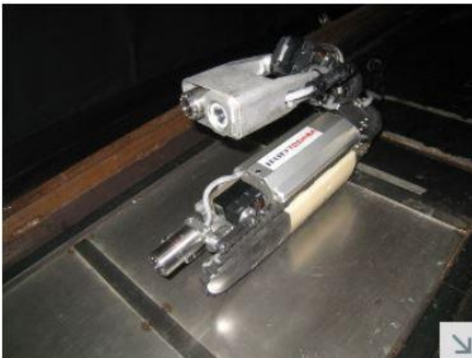
A scorpion-like observation robot scheduled to go into the containment vessel of the No. 2 reactor at the Fukushima No. 1 nuclear plant. (Photo courtesy of Tokyo Electric Power Co.)
