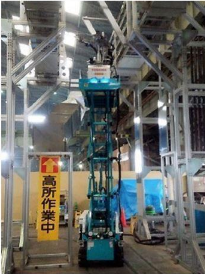
The new cleanup robot is seen extended to its full 8-meter height. (Mainichi)
