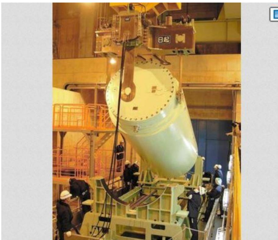
Spent nuclear fuel is kept in a dry cask for storage at the Tokai No. 2 nuclear power plant in Tokai in Ibaraki Prefecture. (Asahi Shimbun file photo)
